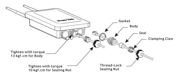
4. Use an adjustable wrench and tighten the thread-lock sealing nut with torque 10 kgf-cm.
