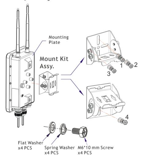
4. Insert the pipe clamp into the mount kit assembly.
