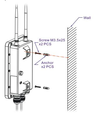
Keep the distance between the screw head and the wall about 10 ~ 15mm.
