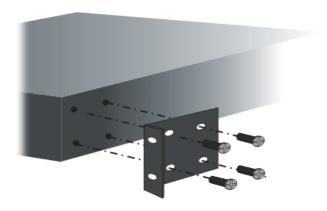
2. Then, install the Vigor router (with rack mount kit) on the 19-inch chassis by using other four screws.
