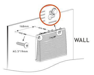
3. When you finished about procedure, the router has been mounted on the wall firmly.
