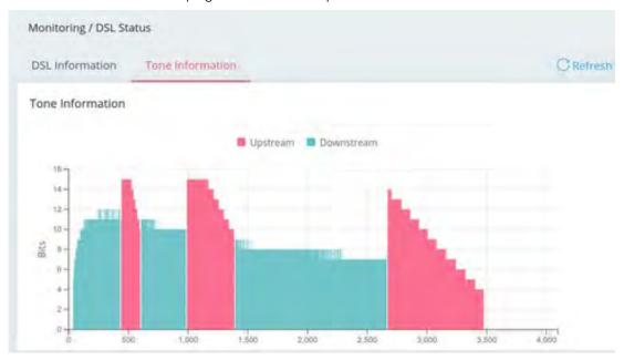
The above figure shows the bandwidth shared between Upstream (Red) and Downstream (Blue).
