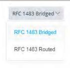
Multiplexing - Encapsulating type of the ADSL connection.
