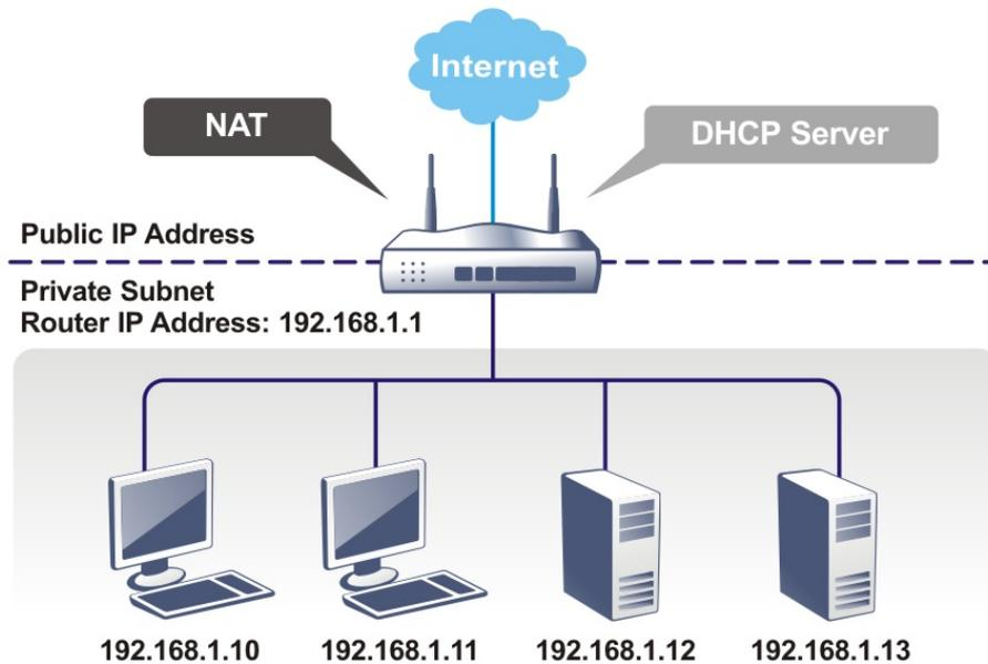
In some special case, you may have a public IP subnet from your ISP such as 220.135.240.0/24. This means that you can set up a public subnet or call second subnet that each host is equipped with a public IP address. As a part of the public subnet, the Vigor router will serve for IP routing to help hosts in the public subnet to communicate with other public hosts or servers outside. Therefore, the router should be set as the gateway for public hosts.
