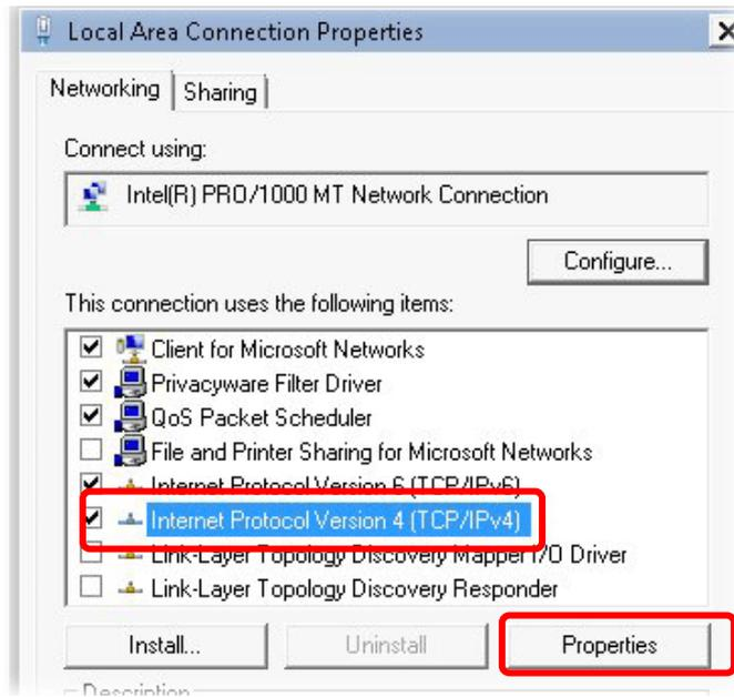
5. Select **Obtain an IP address automatically** and **Obtain DNS server address automatically**. Finally, click **OK**.
