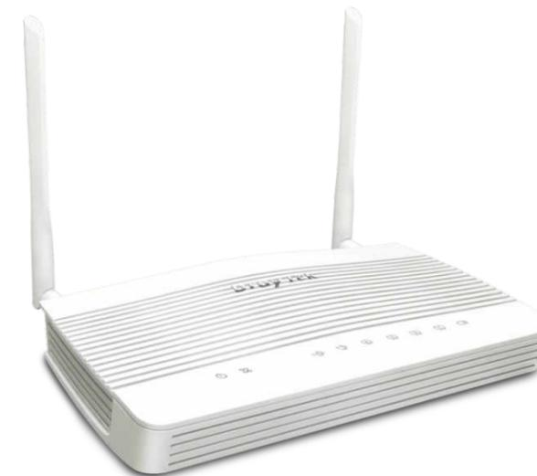
Vigor2767 Series is a VDSL2 35b supervectoring modem, a firewall, and a VPN router. The router has 1x 2.5GbE LAN port which is switchable to be a backup WAN interface. It's highly configurable for an abundance of features including web content filtering, bandwidth limit, QoS and lots more, perfect for professional users who would like to take full control of the network.
