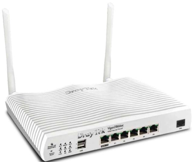
Vigor2866 Series is a dual WAN firewall router. It has one G.fast supported DSL WAN, delivering fiber-like speed up to 1 Gbps, and one configurable Ethernet WAN. The built-in DSL modem is backward compatible with VDSL2 profile 35b supervectoring and ADSL2+. Vigor2866 Series provides load-balancing and failover for your business continuity. Featuring VPN, QoS, route policy, firewall, content filtering, bandwidth management, captive hotspot portal.
