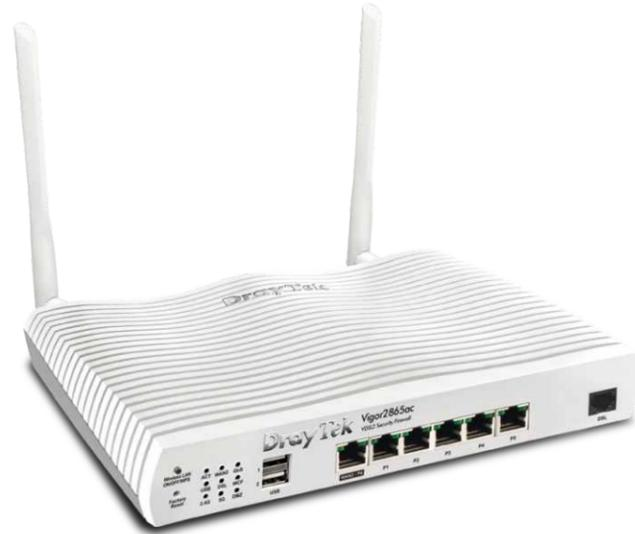
Vigor2865 Series is a VDSL2 35b/ADSL2+ Security Firewall router integrating a DSL modem which is compatible with variants of ADSL and VDSL, including profile 35b supervectoring. There is also a Gigabit Ethernet WAN port for broadband connections to share the traffic load or serve as a failover connection.
