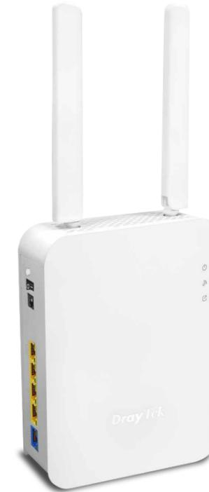
VigorAP 906 is 11ax wall-mount/desktop wireless access point with a 5-port LAN switch. With wire-like link rate up to 2402 Mbps\* in 5GHz band and up to 574 Mbps in 2.4GHz band, it's suitable for high density environments. It can be cloud-managed by VigorACS, and also act as the mesh Root AP to manage up to 7 mesh node APs in LAN.
